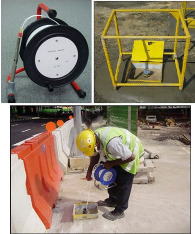
Fig. 22.24 Standpipe and piezometer
