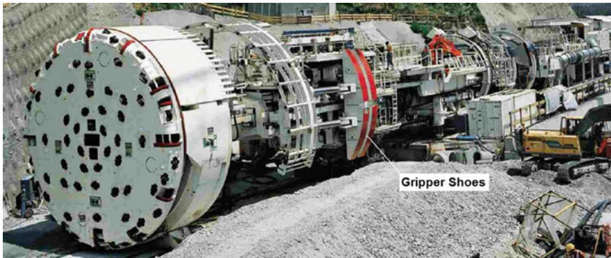
Fig. 14.16 Single-gripper TBM for hard rock (Reproduced by permission of Copyright © 2005, Tunnelseis)
