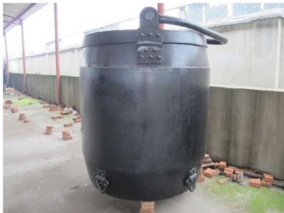
Fig. 19.18 Steel kibble for shaft sinking
