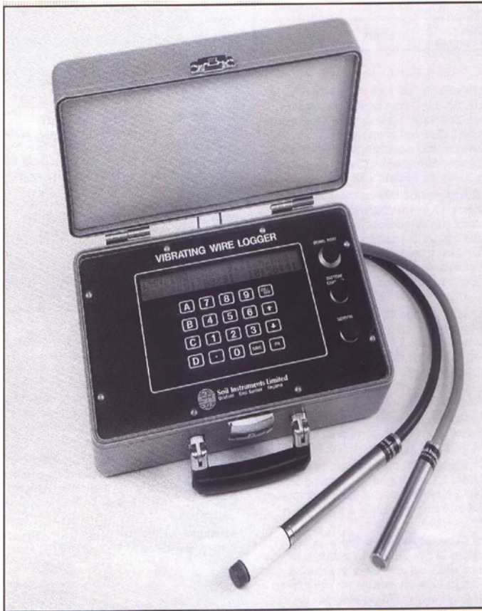
Fig. 22.26 Vibrating wire piezometer. Source http://jatiluhurdam.wordpress.com
