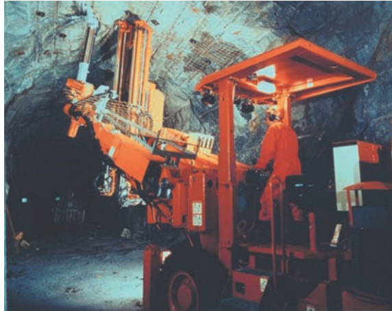
Fig. 21.30 Sandvik Robolt 320 with screen manipulator (Reproduced from Ref. [8] by permission of Sandvik)
