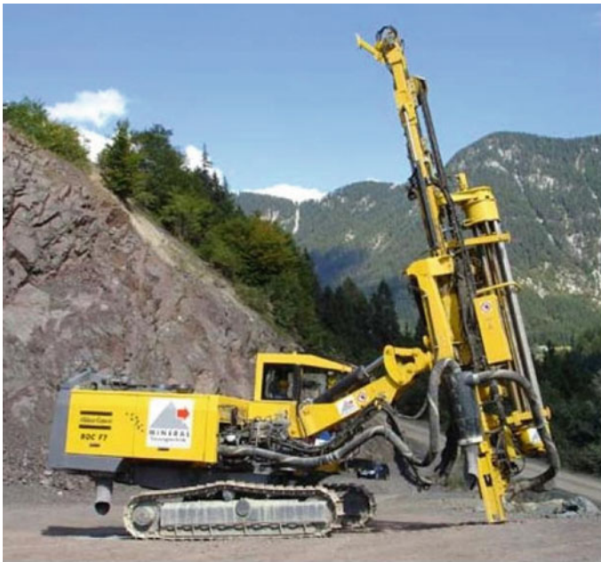
Fig. 2.27 COPROD drill string (Reproduced with the permission from Atlas Copco)
