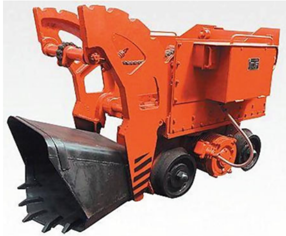
Fig. 19.1 Overhead shovel loader, rail-mounted
