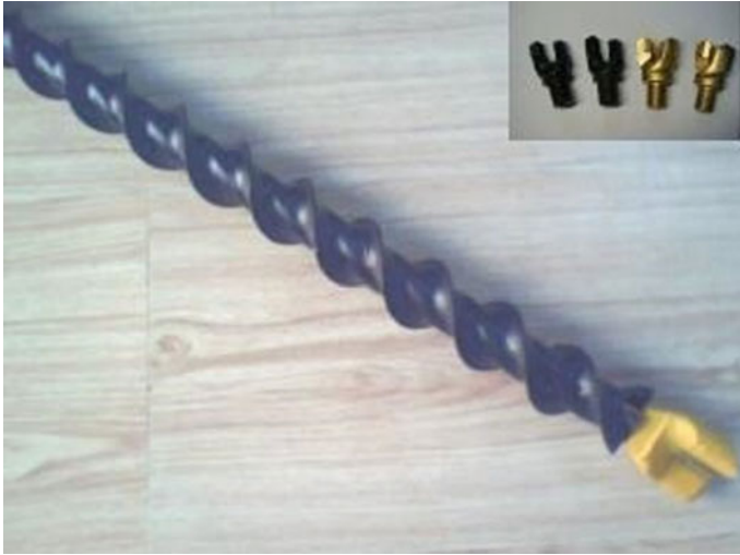
Fig. 2.38 Auger drill with two-wing drag bit
