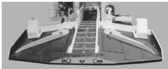
3 Two lateral loading beams
