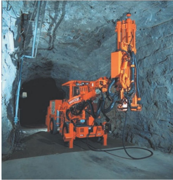
Fig. 21.29 Fully mechanized bolting rig (Reproduced by permission of Sandvik)
