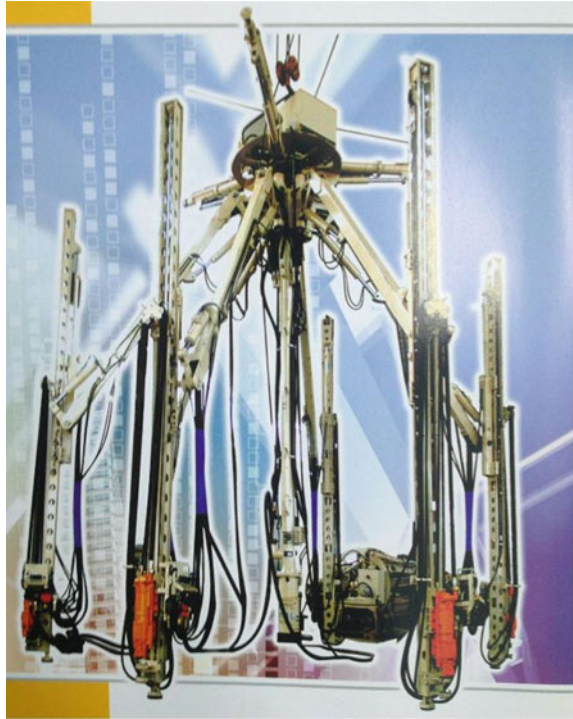
Fig. 16.8 Vertical shaft drill made by Qingtao Grandplan Technology Co. Ltd., China
