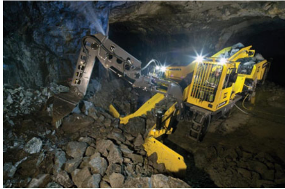
Fig. 19.5 Atlas Copco's continuous loader: Häggloader 10HR/10HR-B
