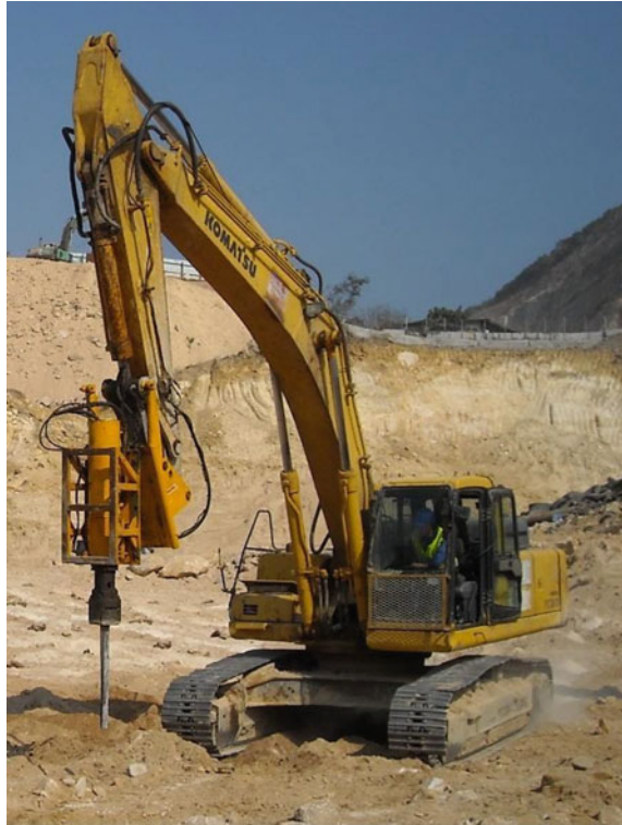
Fig. 7.7 Excavator-mounted hydraulic splitter
