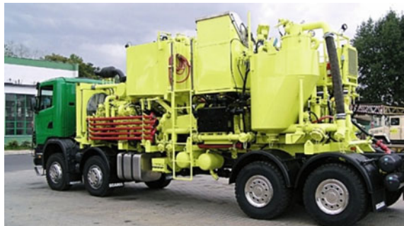
Fig. 21.20 Dwupompowy cementing unit equipped with two Caterpillar engines, two pumps SPM TW 600S, and continuous mixing systems Source http://polskiproducent.pl/
