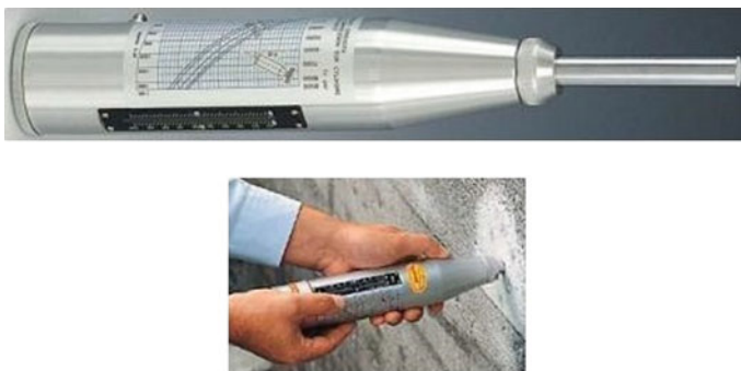
Fig. 1.7 Schmidt Hammer rebound hardness test (Source [10])
