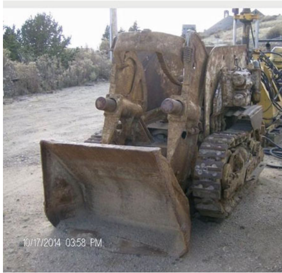
Fig. 19.17 Eimco 630 air mucking machine (Source www.savonaequipment.com/en )
