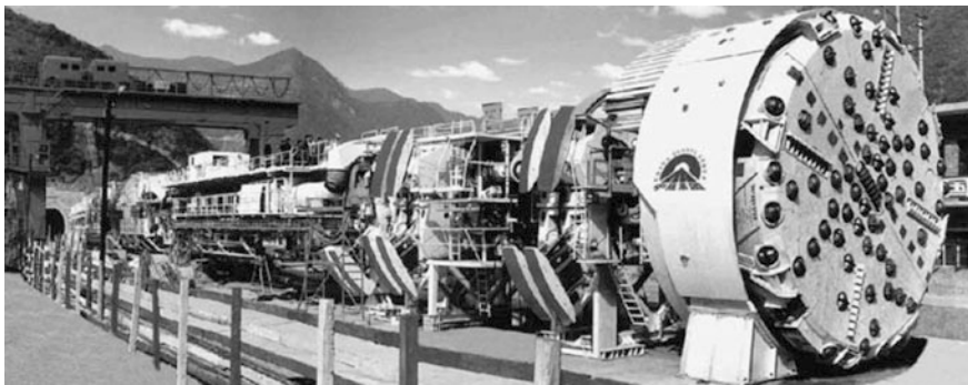
Fig. 14.17 Double-gripper TBM for hard rock, TB880E, Dia. 8.8 m, developed by China Railway Group (Courtesy of Central South University, China)
