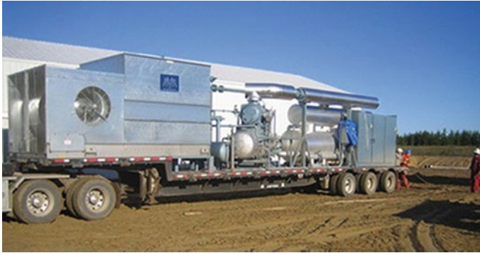
Fig. 21.7 Movable refrigeration unit Source www.mmrefrigeration.com
