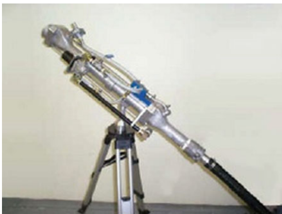
Fig. 16.18 Pneumatic cartridge loaders made by Can-Blast Inc. Source www.can.blast.com/
