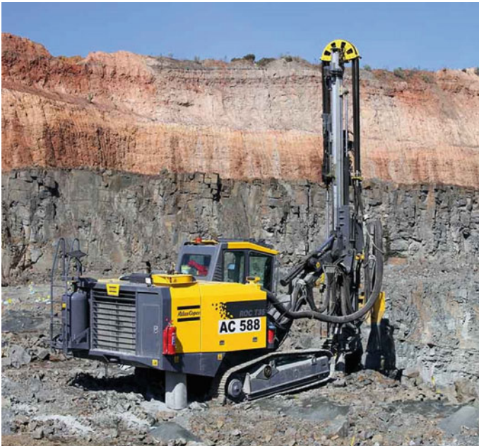
Fig. 2.19 Crawler rig for surface drilling (Reproduced with the permission from Atlas Copco)
