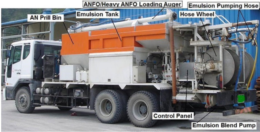
Fig. 3.46 Multi-function mobile manufacture unit (MMU)
