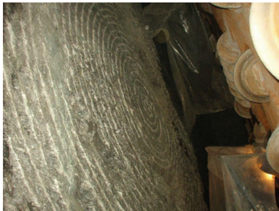
Fig. 14.23 Track of the cutter on the face (Reproduced from http://www.bartz.es/en/contenido/?idsec=517 by permission of Bartz)
