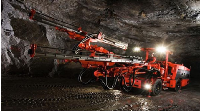
Fig. 2.20 Wheel-mounted rig for underground drilling (Reproduced with permission from Sandvik)
