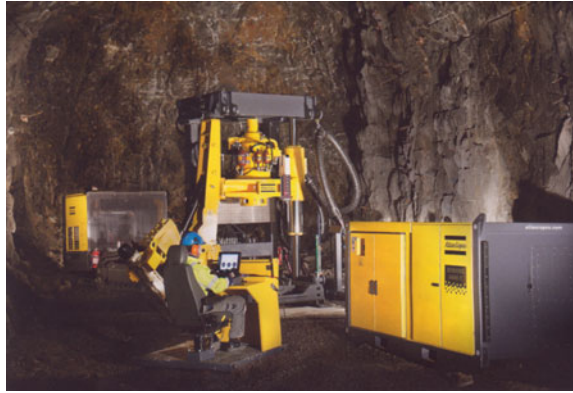
Fig. 14.8 The Robbins 34RH C raise boring machine (Reproduced from Ref. [18] by Permission of Atlas Copco)
